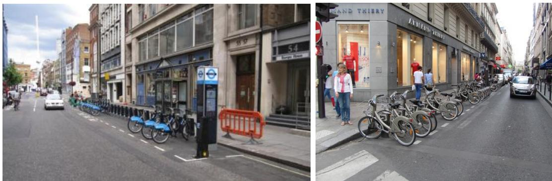
Figure 19. A cycle sharing station can fit in a 2 m wide parking lane, as demonstrated in London (L) and Paris (R).
